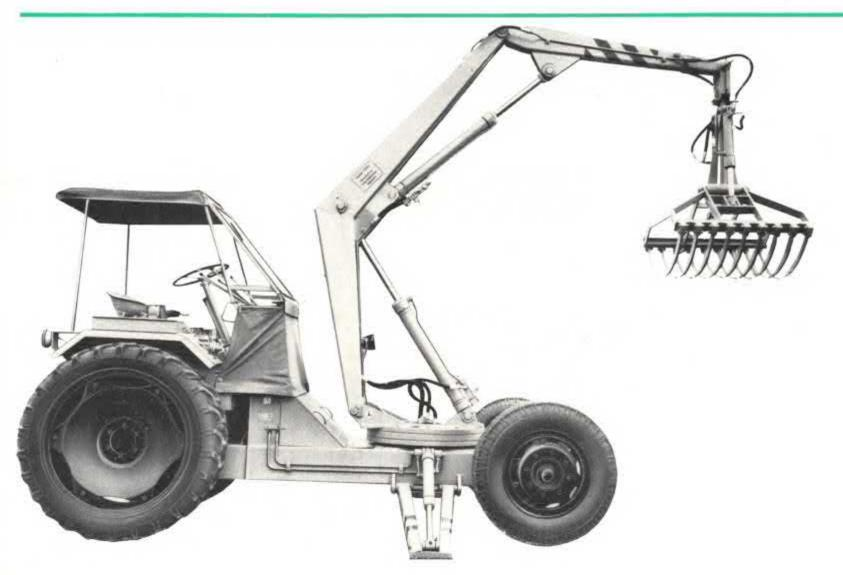
The front axle is attached to a floating joint and will compensate for any uneveness of the ground. As a safety precaution the floating motion is limited. By removing the front cover plate easy access to steering linkage and headlamps is provided. The tow hook is welded to the axial frame tube, and access is provided by an opening in the cover plate.
