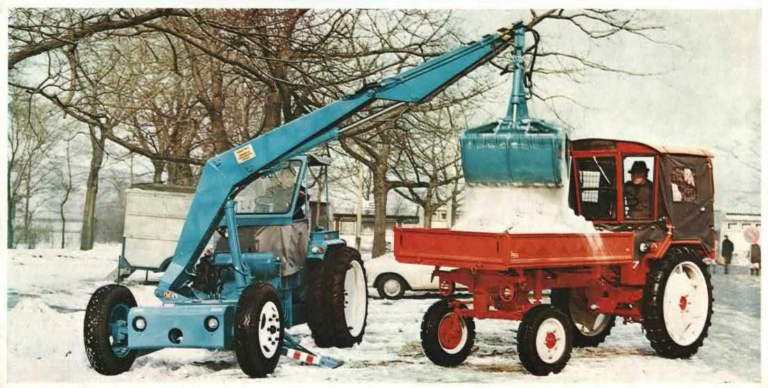
Our combine has developed this loader for agriculture, road construction and for municipal work. As experience shows the 750 kg carrying capacity of our T 157/2 is quite sufficient for these fields of application. Moreover, this carrying capacity is ensured at any jib position. For economic data on this hydraulic multi-purpose loader see page 8 of this brochure.
